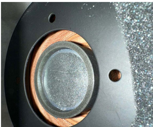
Elaborate: The weight trims the mass and thus the resonance of the passive diaphragm. This is also kept on axis by a centering spider and thus prevented from wobbling
