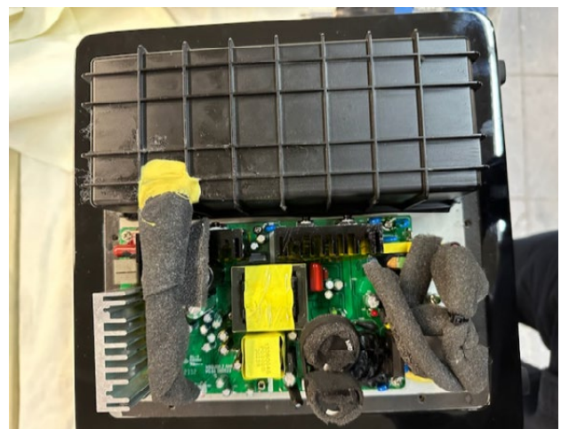
Rear of the electronics: Input and output board as well as the entire DSP section are airtight encapsulated (Photo: Velodyne Acoustics)
