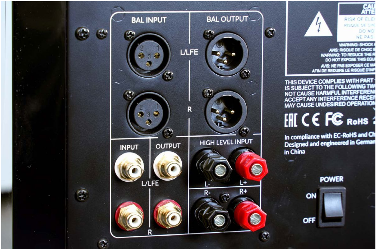
It couldn't be more universal: 2 channels each of XLR and RCA inputs and outputs and parallel connection to speakers (Photo: R. Vogt)
