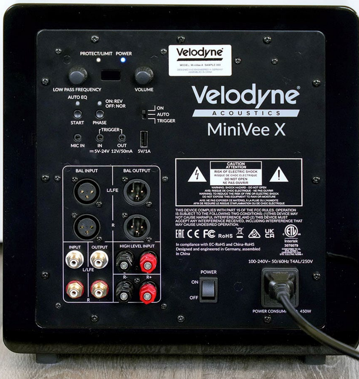
The new generation subwoofer amplifier/processor with Auto-EQ calibration and app control via Bluetooth (Photo: R. Vogt)
