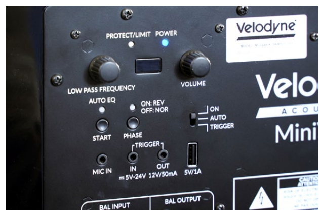
Buttons for auto EQ and phase inversion including indicator light. Clever: Trigger remote activation with 5V from USB and delayed trigger output, for example
