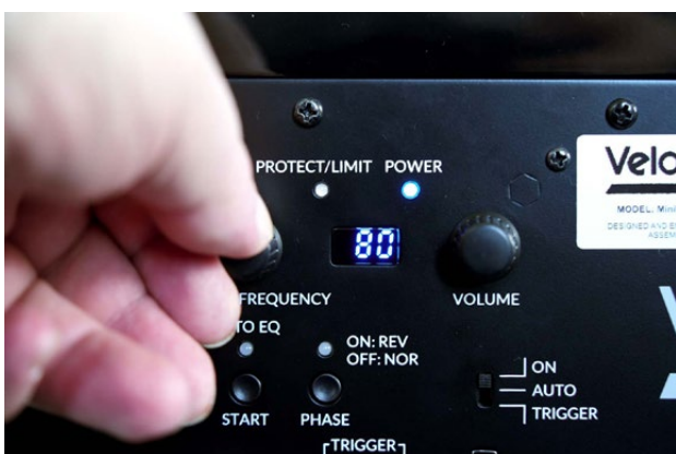
Analog rotary knobs control the upper cut-off frequency and the level; the display shows the respective value
