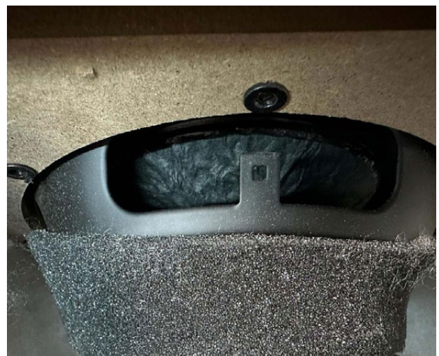
A fixed paper cone transmits the force of the voice coil to the flat carbon fiber cone
