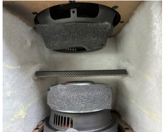
The opposing woofers ensure good force equalization and low cabinet movement. Vertical damping is provided by a strut (Photo: Velodyne Acoustics)
